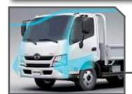
The windshield angle is optimized while the top corners boast a more gradual curve, thereby lowering the Cd (coefficient of drag) value, and resulting in more efficient aerodynamics.
