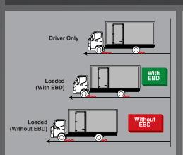
▲ ELECTRONIC BRAKEFORCE DISTRIBUTION (EBD) Optimizes brake force depending on the
