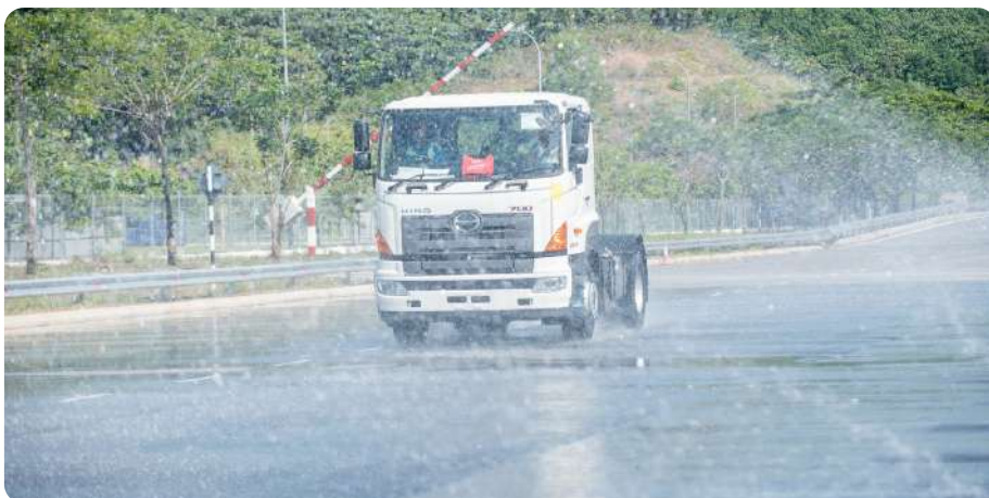
Brake Testing with various conditions
