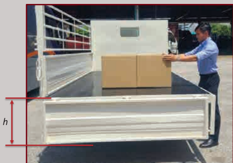
Ground to body floor height, h: 880mm *XZU600 (5t) height: 980mm
