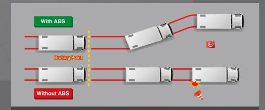
▲ ANTILOCK BRAKING SYSTEM (ABS) An active safety feature designed to help driver retain steering control by preventing wheels from locking up during emergency braking
